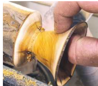
▲ Pic.7 Keep checking the wall thickness with your fingers; if you don't get it thin and fairly even it will make the goblet top heavy
